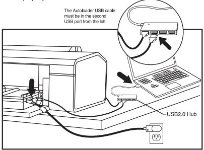
**Note:** Make sure the RoboJet software/driver installation is complete before connecting the Autoloader to the computer.
